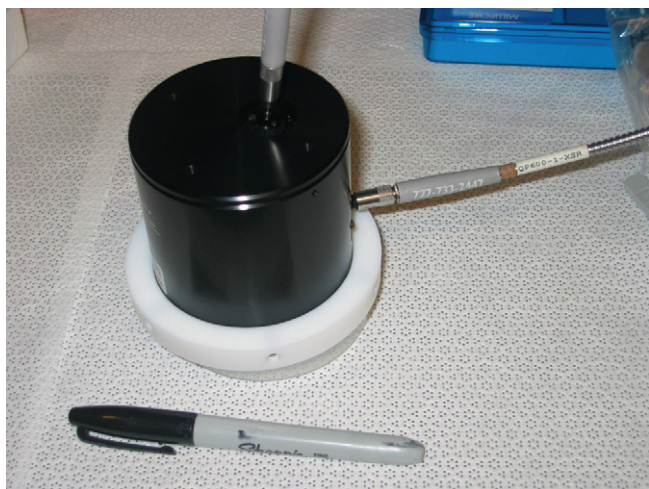
Fig. 1. The modified integrating sphere showing the fiber optical cables with light in at 8^\circ off perpendicular and detector cable at 90^\circ . A reflective white layer of \text{BaSO}_4 was painted onto the bottom flat surface of the integrating sphere to minimize the loss of light interactive with the black enamel. To avoid flaking of this paint over time, a thin translucent layer of white Teflon (1.5 mm) was added to the bottom of the sphere (with a port to allow light in and out).
